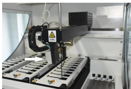
Figure 3.4: Robotic arm, the arrow indicates the scanning module
