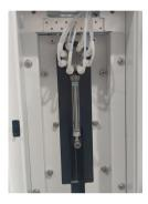
Figure 12.13: Replace the syringe plunger screw
