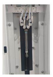
Figure 12.11: Remove the syringe plunger screw (2)
