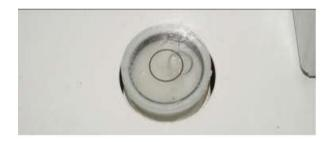
Figure 3.7 Air-bubble level
