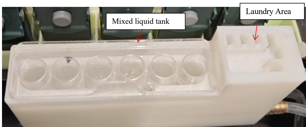
Figure 11: Schematic of washing area and mixing tank
